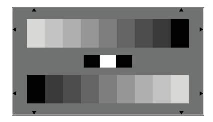
Two 9-graduated counter current gray scales are arranged on a gray background (D = 0.66), the gray scales are graduated according to a gamma of 0.45 (related to the densities).
