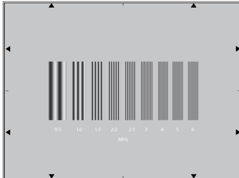
The test chart is designed for measuring horizontal static resolution. It shows vertical bars, the density variation of which gives a sinusoidal video response. This is preferred to a rectangular function test pattern, because this is in fact likely to create harmonic frequencies which can impair resolution measurement owing to know „moirés“ phenomena in CCD Camera. The bars create frequencies of 0.5, 1, 1.5, 2, 2.5, 3, 4, 5, 6MHz.
