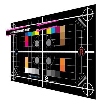
HORIZONTAL SCALES in inch and cm close to the vertical center of the chart. The scale starts with zero in the middle and is symmetrically to both sides of the chart //
