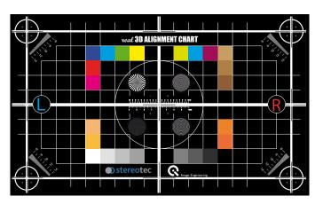
The *real* **3D Alignment Chart** is made to align and adjust cameras for a 3D shooting.
