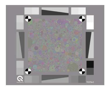
The TE276 V2 Dead Leaves Target is used for the analysis of 'texture loss', which is the loss of low contrast, fine details in images due to noise reduction or other image processing techniques.
