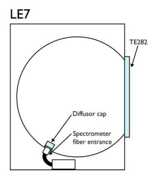
The TE282 D is designed to measure shading/vignetting of a digital camera.
